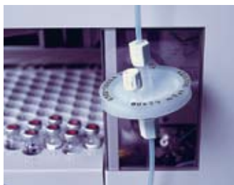
Mobile phase filtered inline using the Aqueous/Solvent IFD device.
