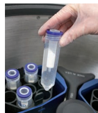
Fig 5. Spin adapters are used together with PD-10 Desalting Columns, PD MidiTrap G-25, and PD MiniTrap G-25 to enable use in a standard centrifuge.
